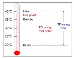
• Condenser capacity stated at the midpoint will be lower than at the dew point.
