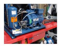
The test rig is an industry standard air cooled condensing unit coupled with DX evaporator, an example is shown in the photo.
