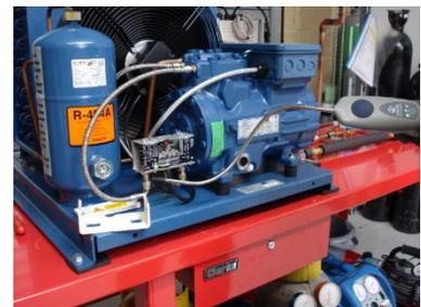
The test rig is an industry standard air cooled condensing unit coupled with DX evaporator, an example is shown in the photo.
