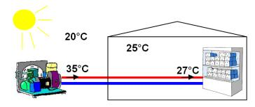
condenses at 35°C. Although the inside (room) temperature is warmer than ambient, it is below the condensing temperature, so the refrigerant subcools. In the example the degree of subcooling is 8K.
