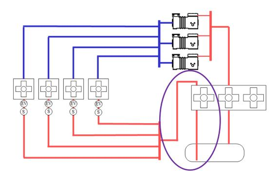
Additional subcooling can also be achieved by using a mechanical subcooler (heat exchanger) in which some of the liquid is expanded and cools the main liquid line.
