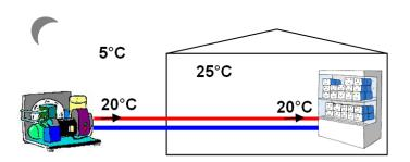
temperature. The refrigerant arriving at the expansion device will be a mixture of liquid and gas (flash gas), so it will have less capacity to absorb heat when it flows through the evaporator. It is not uncommon for this situation to occur, but it has an adverse impact on the performance of the system. Insulating the liquid line inside the building will reduce the amount of flash gas in the liquid arriving at the expansion device.
